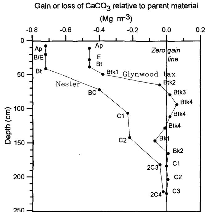
Fig. 3. Volumetric carbonate content (gravimetric content  $\times$  bulk density) of sampled horizons of the Nester and Glynwood taxadjunct pedons. Dots represent the midpoint of each horizon.
