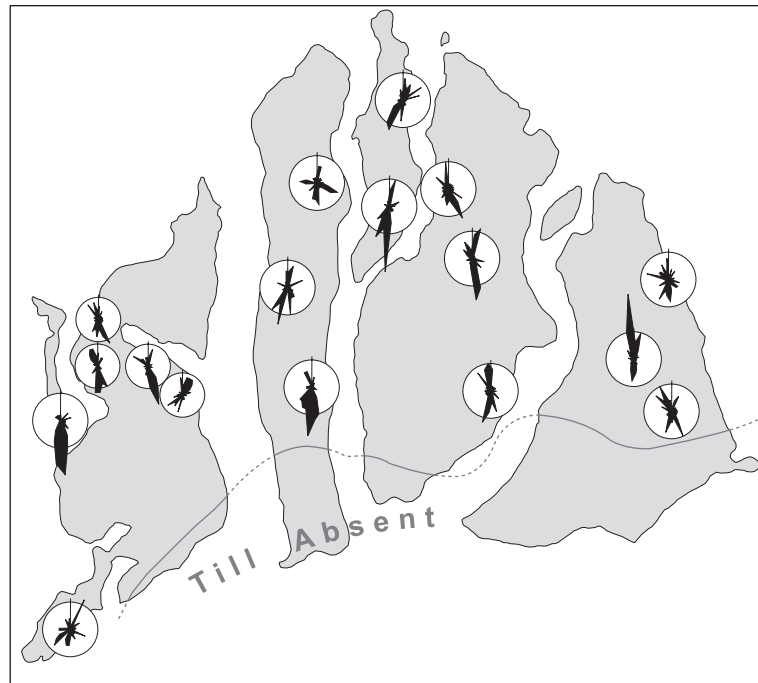
Fig. 11. Rose diagrams showing the till fabric for several sites within the Grayling Fingers. Each diagram is based on a count of at least 50 elongate stones.
