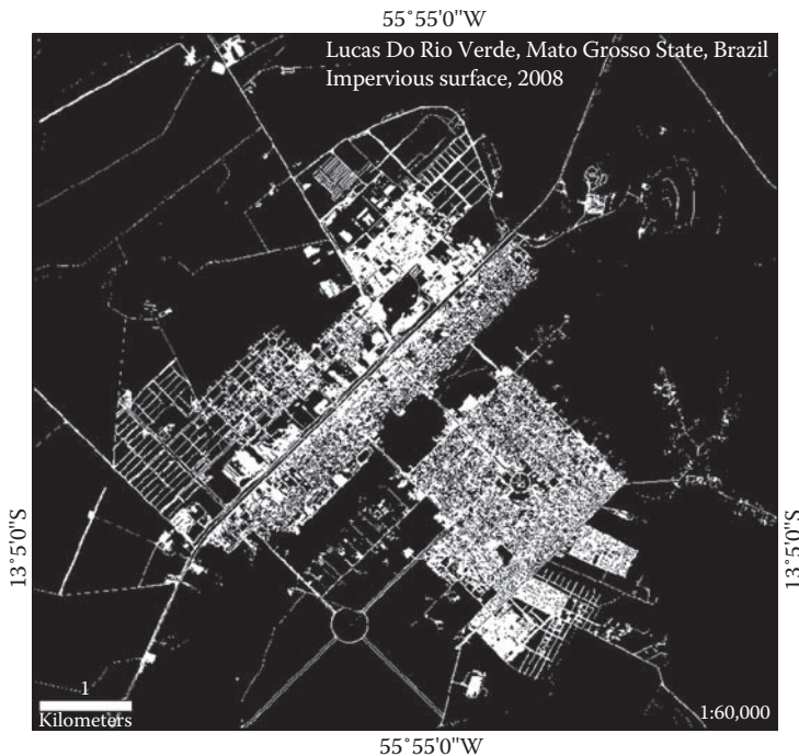
FIGURE 13.6 Impervious surface image developed from QuickBird imagery.
