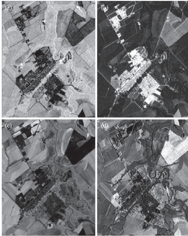
FIGURE 13.7 Fraction images developed with linear spectral mixture analysis based on Landsat TM multispectral data: (a) low-albedo, (b) high-albedo, (c) vegetation, and (d) soil.
