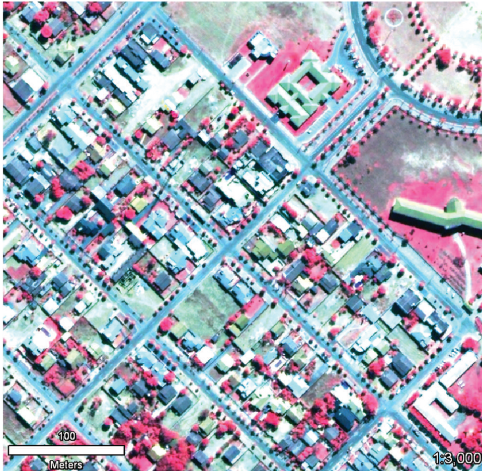
Plate 1. Image false color composite consisting of QuickBird bands 4, 3, and 2 by assigning as red, green and blue respectively, showing the complexity of land-use/land-cover features in the high spatial resolution image
