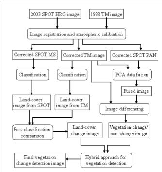
Figure 2. Strategy for vegetation change detection based on Landsat TM and SPOT HRG data. (Note: MS: multispectral image, PAN: SPOT panchromatic image, and PCA: principal component analysis)
