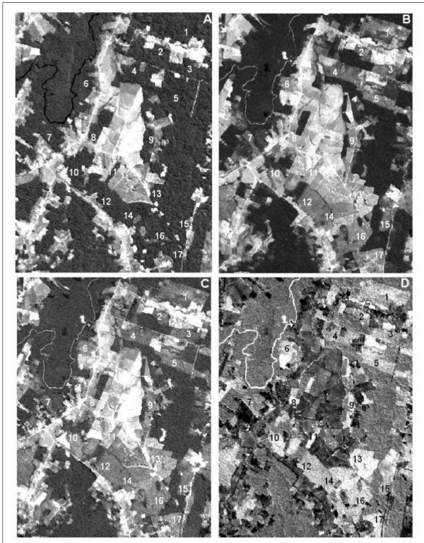
Figure 6. A comparison of change detection results: (a) TM band 5 image in 1998, (b) SPOT panchromatic image in 2003, (c) band 5 image after data fusion, and (d) difference image between fused band 5 and original TM band 5.
