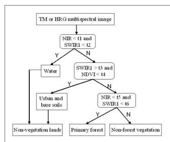
Figure 4. A rule-based approach for land-cover classification. (Note: NIR represents near-infrared, and SWIR1 represents the shortwave infrared band, i.e., band 5 in TM data or band 4 in HRG data; NDVI represents the normalized difference vegetation index; and t1 through t6 represent the thresholds developed from sample plots.)
