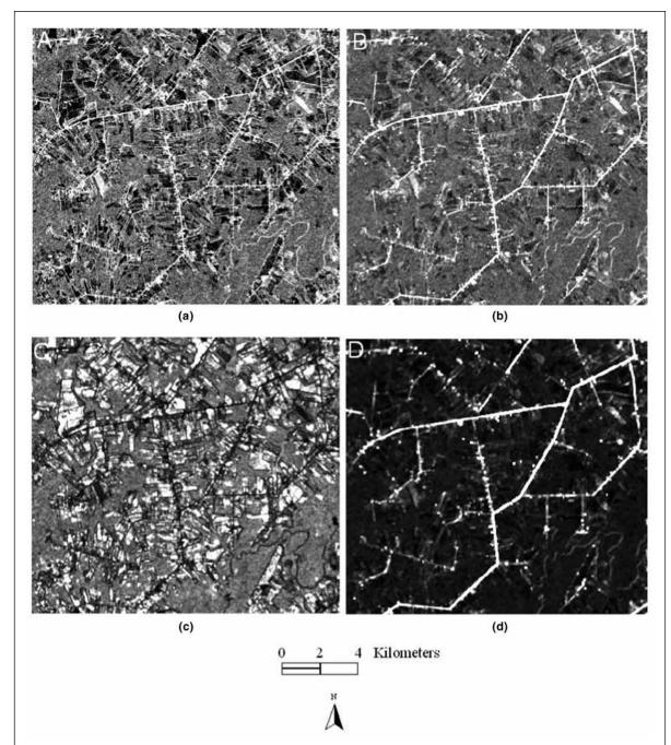
Figure 4. Comparison of selected four textural images with corresponding window sizes based on the SPOT HRG panchromatic image (part of the study area): (a) entropy texture measure with  $9\times 9$  window size, (b) dissimilarity texture measure with  $15\times 15$  window size, (c) second moment texture measure with  $11\times 11$  window size, and (d) contrast texture measure with  $25\times 25$  window size.
