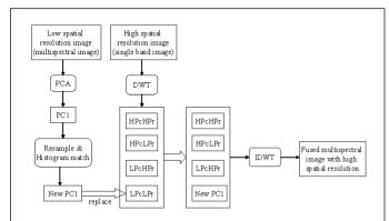
Figure 3. Wavelet-merging approach based on multiple spatial resolution images (PCA and PC1 represent principal component analysis and the first principal component, DWT and IDWT represent discrete wavelet transform and inverse discrete wavelet transform, HP and LP represent high pass and low pass, and c and r represent column and row decimation)
