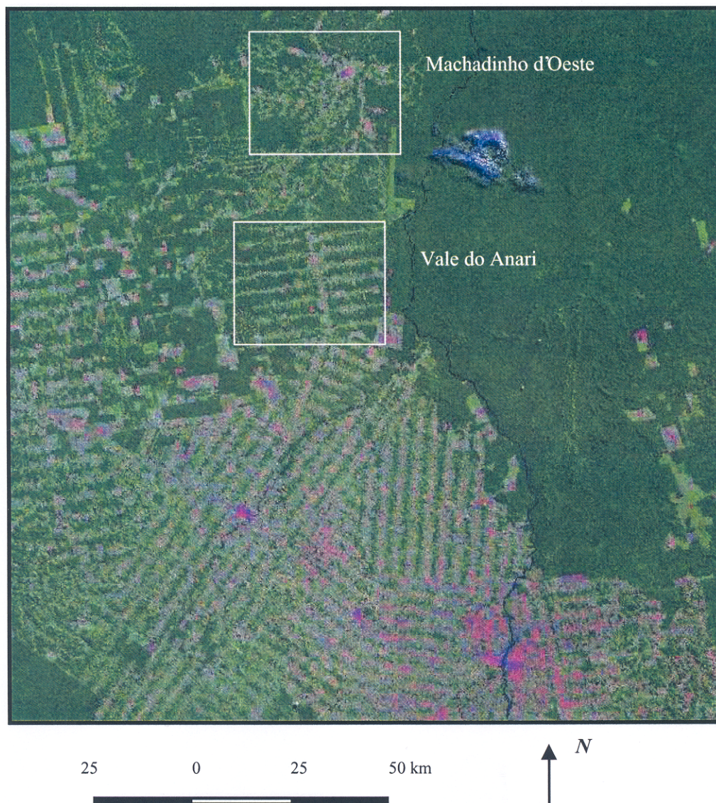
Figure 2. Landsat TM scene showing the orthogonal road network ('fishbone'), including Vale do Anari, and the different settlement design of Machadinho d'Oeste in Rondônia, Brazilian Amazon.
