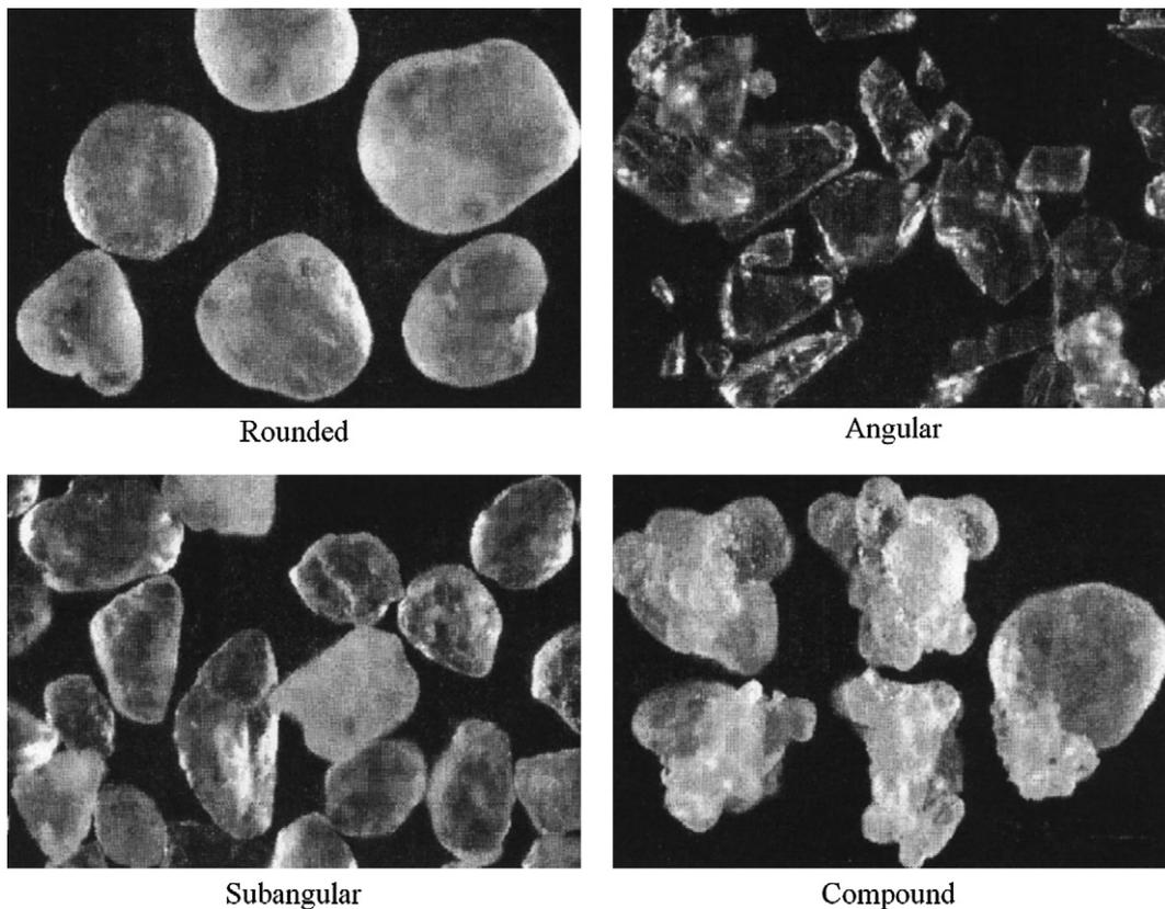
Fig. 6. AFS standard comparison grain shapes used in grain shape determination (modified from American Foundry Society, 2004).
