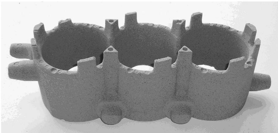
Fig. 2. Foundry sand core used for casting engine block components.
